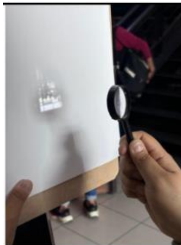
Fig. 4. Use of a magnifying glass as an optical projector.
