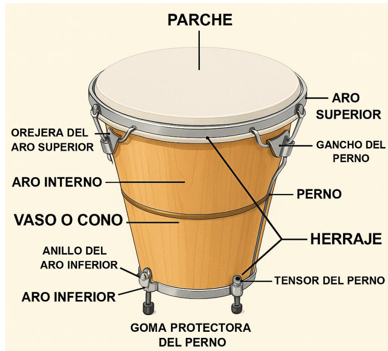
Figure 11. Physical Parts of the Vallenata Box.
