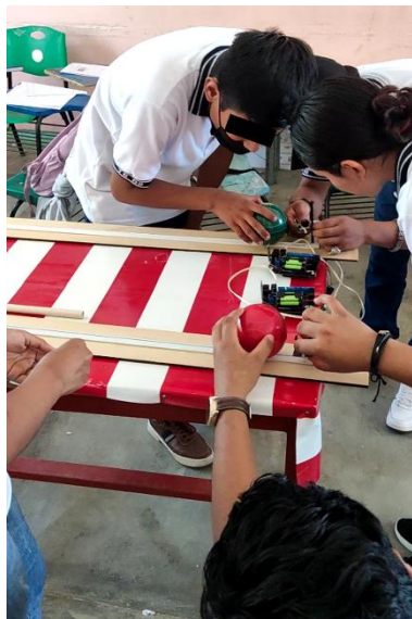
Fig. 8. Students Modifying the Experimental Setup by Adjusting the Height of the ToF Sensor
