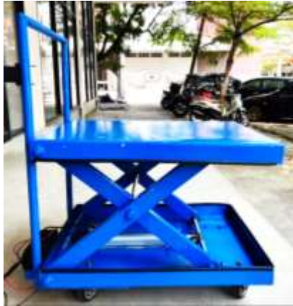
Figure 6: Trolley Utilizing a Linear Actuator Motor for Movement
